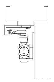
DOOR CLOSER MODELS: 8616 A08P PARALLEL ARM INSTALLATION (PUSH SIDE MOUNT) WITH PLATES DP86, DP86FC
